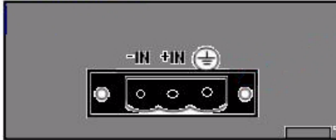
75W, -54.5VDC PoE Power Brick
